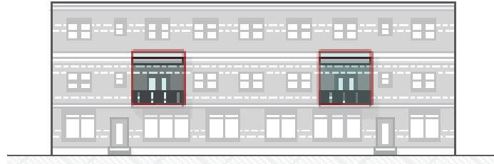
Figure 4.23-10: Articulation with Balconies
